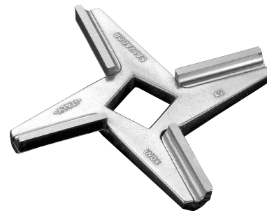
Bimetallic knife mod. "SALVINOX" with braze welded HSS straight inserts mod. 22 - h 13,00 mm mod. 32 - h 13,7 mm mod. 42 (52) - h 18,7 mm
